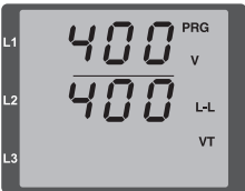
Fig.: Programming mode voltage transformer: The primary and secondary currents can be changed using buttons 1 and 2.
