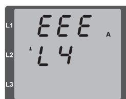
Fig.: Indication of the overrange in current path I4.
