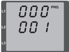
Fig.: Programming mode parameter display: The individual parameters can be changed using buttons 1 and 2.
