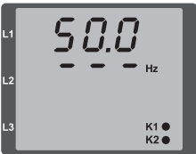
Fig.: No rotation field direction detectable.
