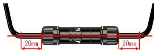
Right way for the cable
