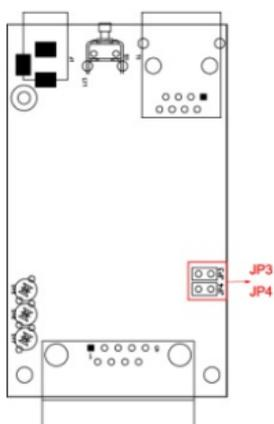
Jumpers are used to set the pull high/low resistor values. The default is 150 K $\Omega$ . Short the jumpers to set this value to 1 K $\Omega$ . Do not use the 1 K $\Omega$  setting with RS-232 mode, since doing so will degrade the RS-232 signals and shorten the communication distance.
