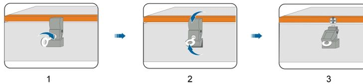
**step 2** Unclip the top and bottom clips of the cabinet.
