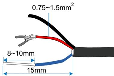
4. Attach appropriate cold-pressed terminals to the stripped wires and crimp them using a crimping tool.
