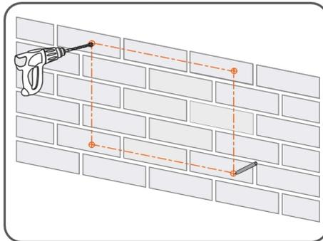
**step 3** Place the M10x45 expansion sleeve (not included in the scope of delivery) into the hole, and tap it with a rubber hammer. Make it completely embedded in the wall.
