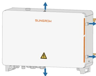
**step 3** Disconnect the upstream input switch of the device, and turn the power switch inside the device to the "OFF" position to ensure the device is voltage-free.
