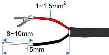
3. Crimp cold-pressed terminals onto the wires.
