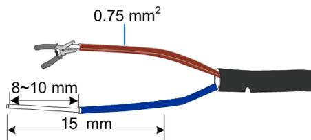
**step 4** Attach appropriate cold-pressed terminals to the stripped wires and crimp them using a crimping tool.
