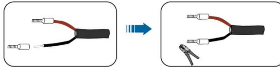
**step 5** Connect the wires to the corresponding positions.
