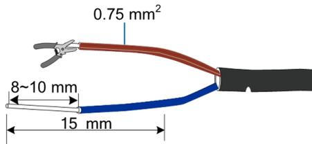
**step 2** Attach appropriate cold-pressed terminals to the stripped wires and crimp them using a crimping tool.
