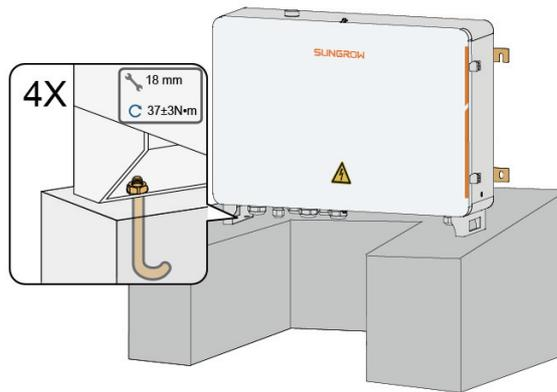
**step 3** Secure the installation holes in bottom of the device to the foundation.
