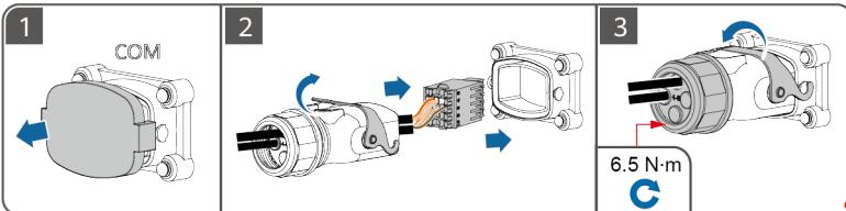
EN Connecting DC Input Power Cables
