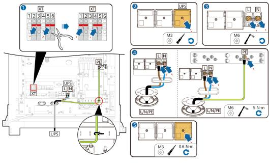
Figure 7-4 Connecting UPS cables
