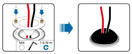
**Step 4** Reinstall the cable baffle plate.
