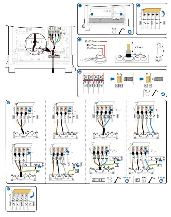
Figure 7-1 Installing PCS power cables
