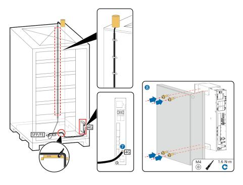
Figure 7-10 SmartLogger cable connection 2
