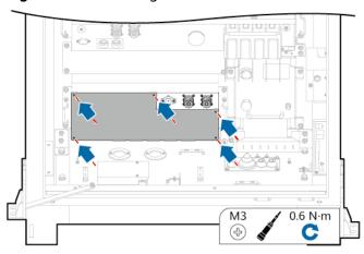
Figure 7-16 Installing the RCM cover
