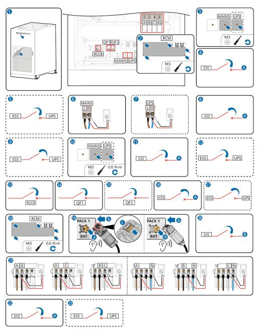
A: Auxiliary power supply switch of the customer's power distribution cabinet
