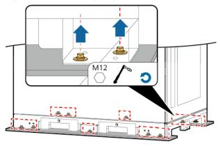
**Step 4** Remove the forklift positioning plates.
