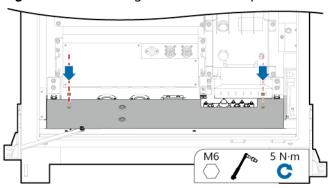
**Step 5** Reinstall the external bottom baffle plate for the ESS.
