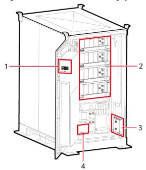
Figure 2-12 Positions of monitoring system components
