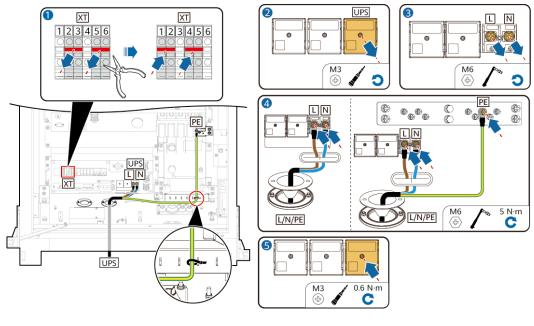
Figure 7-4 Connecting UPS cables
