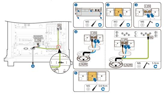
Figure 7-3 Connecting the auxiliary power supply cable (power supply connected to the PCS terminal inside the cabinet)
