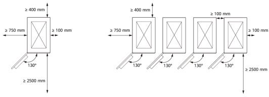
Figure 5-2 Clearance requirements (2)
