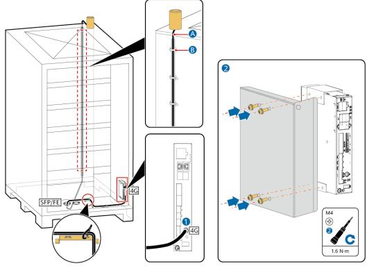
Figure 7-10 SmartLogger cable connection 2
