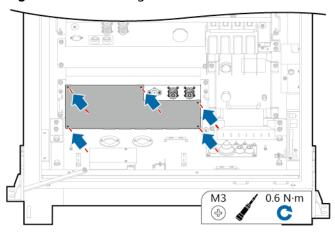
Figure 7-16 Installing the RCM cover
