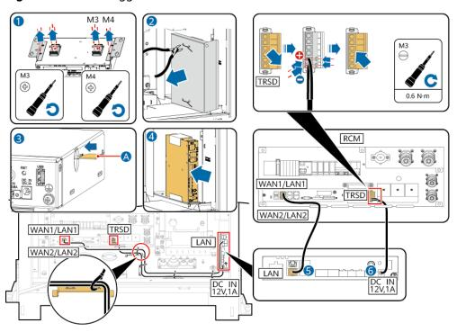
Figure 7-9 SmartLogger cable connection 1
