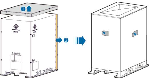
Figure 6-1 Removing outer packaging
