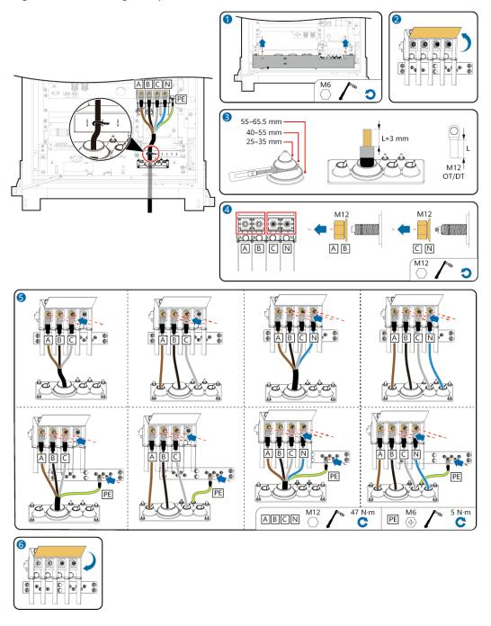
Figure 7-1 Installing PCS power cables
