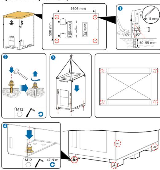
Figure 6-9 Securing the ESS using hidden bolts
