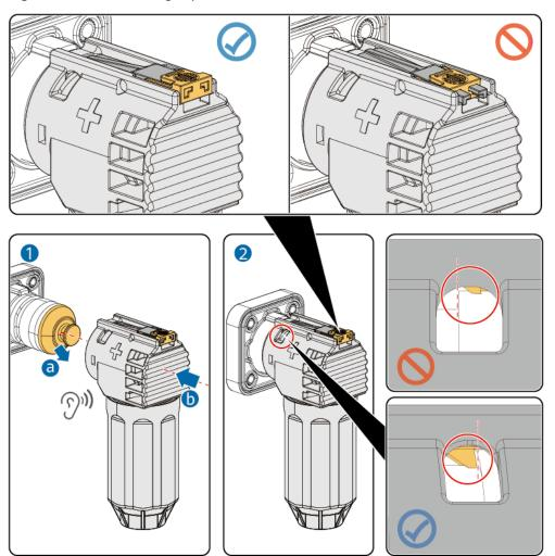
Figure 7-13 Connecting a power cable terminal (model 2)
