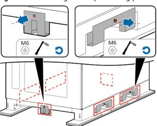
Figure 6-3 Removing forklift positioning plates
