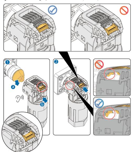
Figure 7-12 Connecting a power cable terminal (model 1)
