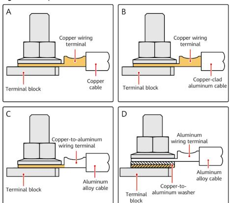
Figure B-1 Requirements on an OT or DT terminal
