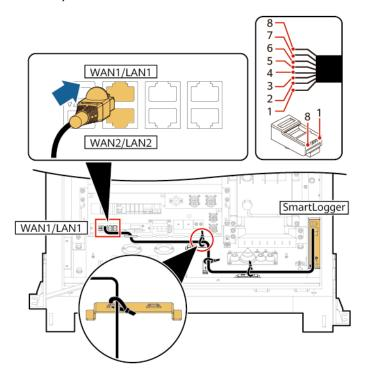
**Figure 7-6** Connecting communications cables (for the SmartLogger installed outside the ESS)
