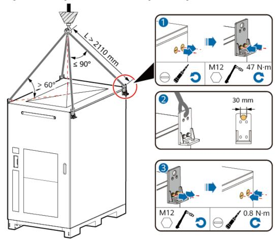
Figure 6-4 Moving the ESS (method 1: using bridle slings)
