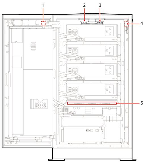
Figure 2-20 Position of the thermal runaway suppression system
