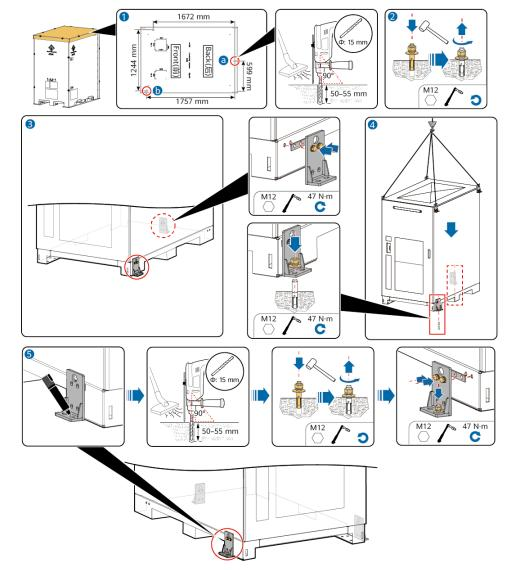
Figure 6-8 Securing the ESS using three anchor brackets
