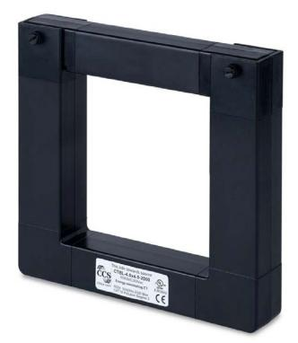
The CTBL series of bus bar current transformers measure current in large conductors. They are UL Listed with a 0.33333 Vac (333.33 millivolt) AC output.
