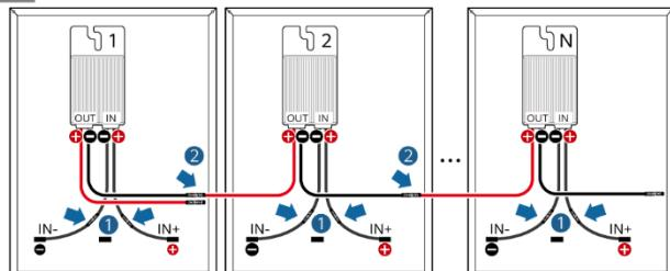
**EN-GB** Connect optimiser inputs to PV modules and connect optimiser outputs to form a PV string.
