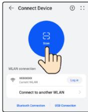
**EN** Log in to the FusionSolar app as an installer, choose Services > Commission Device, and connect to the WLAN hotspot of the inverter.
