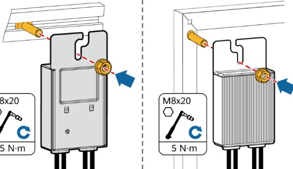
**EN-GB** Installation using a bolt assembly
