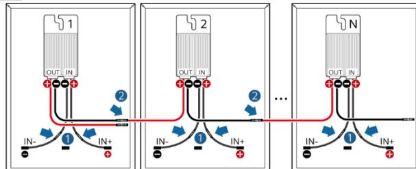
**EN** Connect optimizer inputs to PV modules and connect optimizer outputs to form a PV string.
