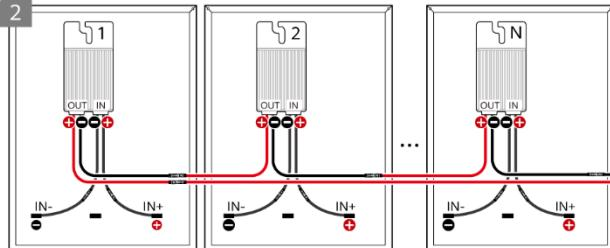
**EN-GB** When the PV string voltage is less than 1 V, measure the PV string resistance and ensure that  $(R1 + R2)/2 \text{ k}\Omega \approx N \times 1 \text{ k}\Omega$ . For example, if a PV string has 16 optimisers, the PV string resistance should be about 16 kΩ.
