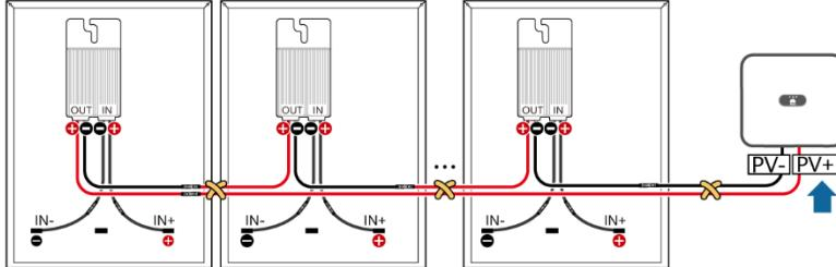
**EN-GB** Determine PV string cable polarity.
