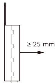
**EN-GB** Ensure that each PV module in the PV string is equipped with an MERC-600W-PA0 optimiser. The figure shows the recommended installation clearances.
