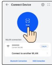
**EN-GB** Log in to the FusionSolar app as an installer, choose Services > Commission Device, and connect to the WLAN hotspot of the inverter.
