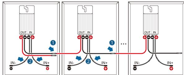
**EN-GB** Connect optimiser outputs to form a PV string, and connect optimiser inputs to PV modules.
