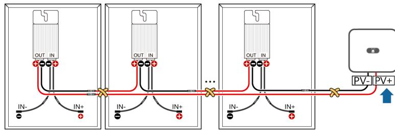
**EN-GB** Connect the PV string to the inverter only after ensuring that the PV string voltage is correct. Otherwise, optimisers may be damaged. It is recommended that the distance between the positive and negative cables of optimisers be minimised.
