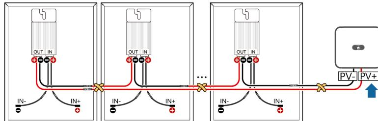
**EN** Connect the PV string to the inverter only after ensuring that the PV string voltage is correct. Otherwise, optimizers may be damaged. It is recommended that the distance between the positive and negative cables of optimizers be minimized.
