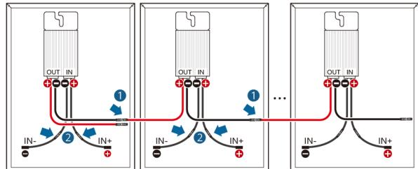
EN Connect optimizer outputs to form a PV string, and connect optimizer inputs to PV modules.
