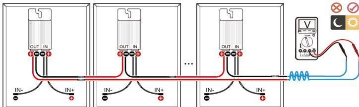
**EN** Use a multimeter to measure PV string voltages. The voltage of each PV module shall be 1 V (tolerance:  $\pm 5\%$ ), and the voltage value (tolerance:  $\pm 5\%$ ) of the PV string shall be equal to the number of optimizers in the string. If the probes are reversely connected, the voltages measured are negative values. If PV string voltages are abnormal, check the cable connections by referring to the user manual.
