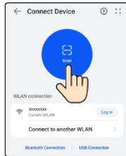
**EN** Log in to the FusionSolar app as an installer, choose **Services > Commission Device**, and connect to the WLAN hotspot of the inverter.
