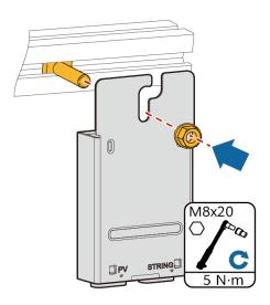
Method 2: Install the optimizer to the PV module frame using a bolt assembly.
