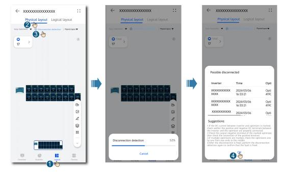
Figure 4-1 Optimizer disconnection detection
