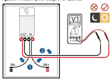
Figure 6-1 Measuring the voltage of an optimizer
