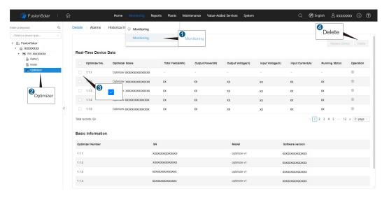
**Step 2** After deleting the old optimizer, update the physical layout. The physical layout must be configured for optimizers. When an optimizer is faulty, it can be quickly located and replaced based on the physical layout. For details, see the **FusionSolar Physical Layout User Guide**.
