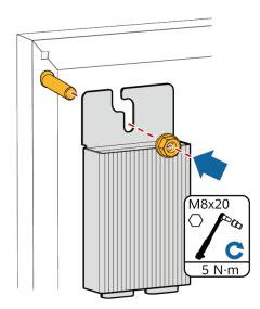
Method 3: Install the optimizer to the PV module frame using a frame mounting bracket (front installation).
