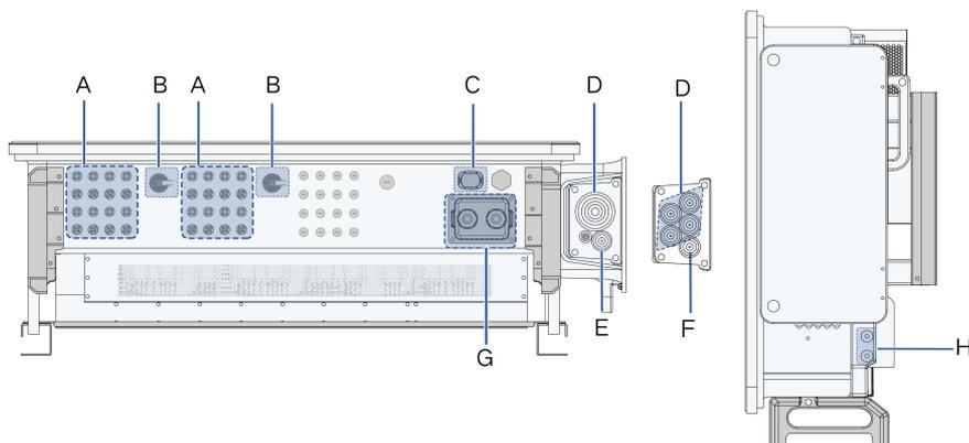
figure 5-2 Description des bornes (SG75CX-P2)
