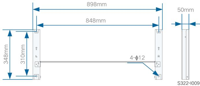
figure 4-1 Dimensions du support de montage
