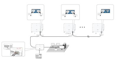
**figure 5-7** Multi-inverter Communication System 【RS485\_1 interface (RJ45)】
