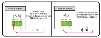
figure 5-8 Normally open contact
