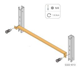
step 2 Level the assembled mounting-bracket by using the level, and mark the positions for drilling holes.
