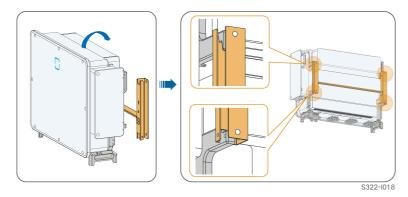
step 3 Fix the inverter with screws.
