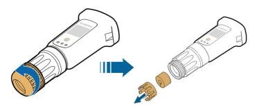
step 3 Unscrew the housing from the communication module.
