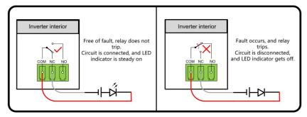
figure 5-9 Normally closed contact
