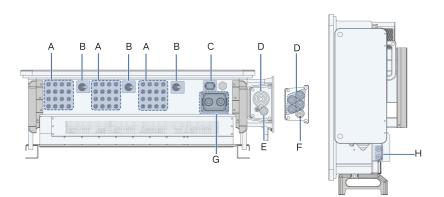
figure 5-1 Terminal Description(SG125/110CX-P2)
