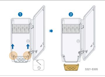
The screws on the sealing plate are captive screws. When the sealing plate is removed, the screws remain on it.
