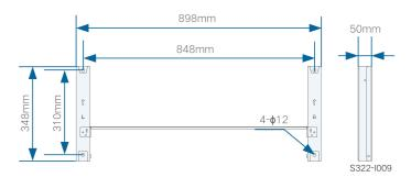
figure 4-1 Dimensions of Mounting-bracket
