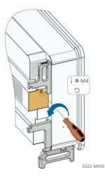
step 3 Press the tab of the latch hook, unplug the cable connection joint outwards, and loosen the screw on the fan holder.
