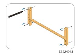
**step 3** Insert the expansion bolts into the holes and secure them with a rubber hammer. Fasten the nut with a wrench to expand the bolt. Remove the nut, spring washer, and flat washer, and store them properly.
