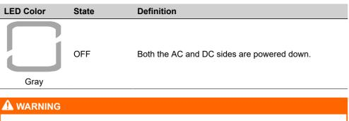
Voltage may still be present in AC side circuits after the indicator is off. Pay attention to the electricity safety when operating.
