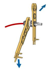
step 5 Check for polarity correctness.
