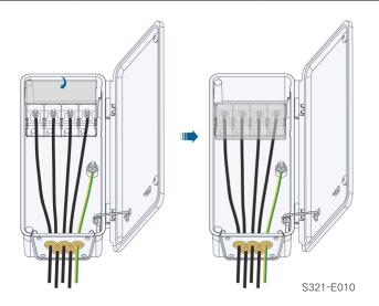
step 9 Remove the limit rod and put it back. Close the junction box and tighten the two screws on the front cover using the supplied hexagon socket wrench.
