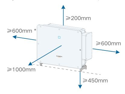
\* In case this distance is less than the distance in the diagram, move the inverter from the mounting-bracket or wall before maintaining fans.
