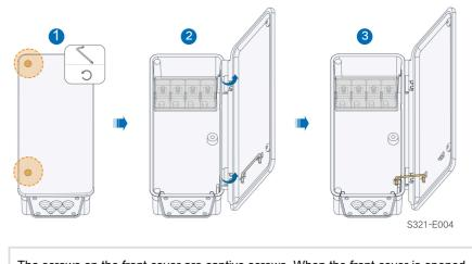
The screws on the front cover are captive screws. When the front cover is opened, the screws remain on it.
