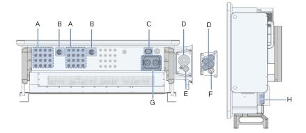
figure 5-2 Terminal Description(SG75CX-P2)
