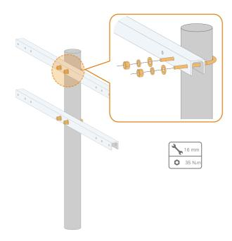
step 5 Use bolts to secure the mounting-bracket to the U-beam.
