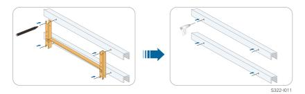
step 3 Secure the mounting-bracket with bolts.
