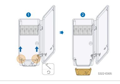
The screws on the sealing plate are captive screws. When the sealing plate is removed, the screws remain on it.
