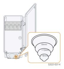
step 3 Lead the cable through the seal ring. The length of unstripped cable in the AC junction box is 50mm.
