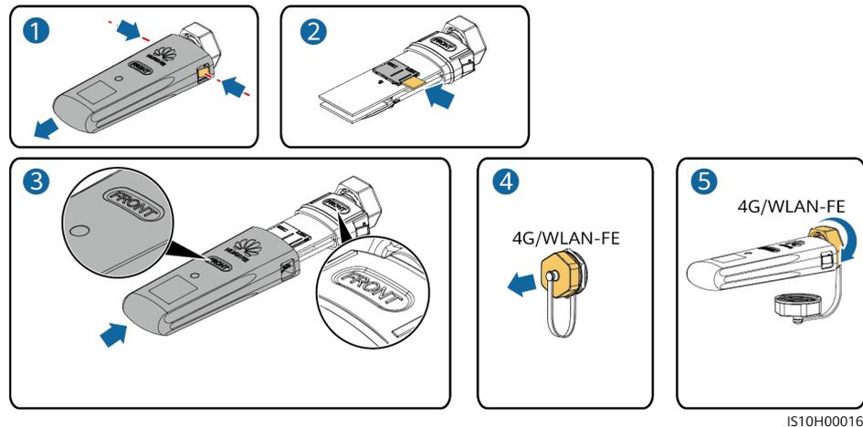
**Figure 5-15** Installation du Smart Dongle 4G (SDongleB-06)
