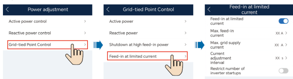
Figure 7-8 Feed-in at limited current
