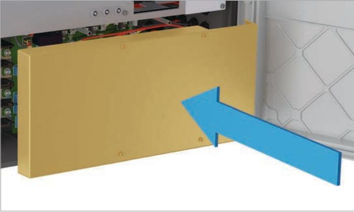
6. Mount and screw on the cover of the AC surge protection devices.
