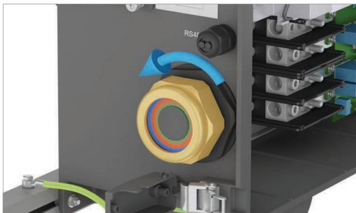
1. Unscrew the cable gland for the AC connection, remove the cable gland and seal.
