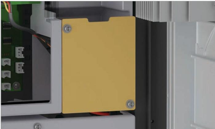
The fan module is located on the left side of the inverter.
