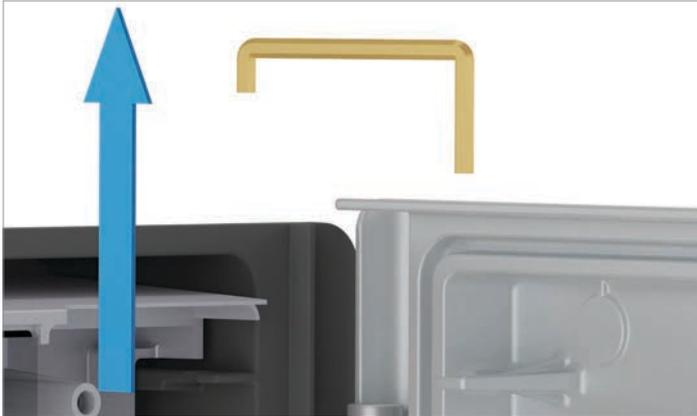
1. Remove the Allen key from the top of the door.
