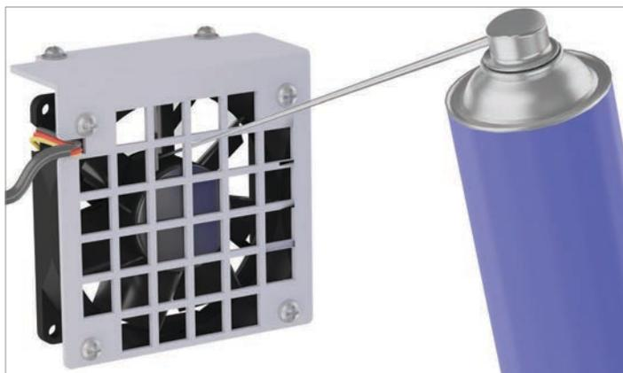
4. Clean the fan and metal housing with compressed air or a firm brush.
