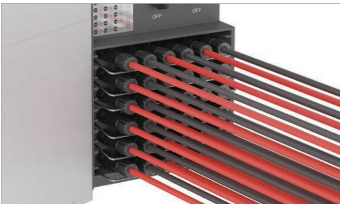
4. The illustration on the left shows how the wiring should look when all DC connections are in use.
