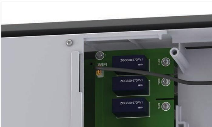
3. Thread the cable through the cable gland and seal.
