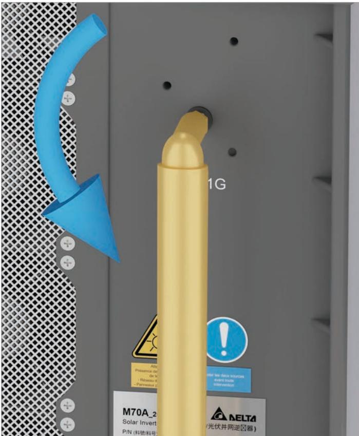
6. Rotate the Sub-1G antenna downward.
