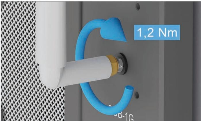
5. Mount the new Sub-1G antenna and screw it on so that it can still be rotated.
