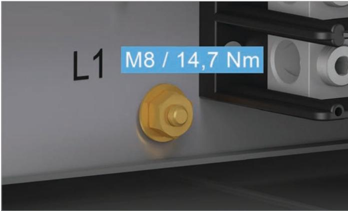
1. Screw the PE/PEN cable onto the PE screw (torque: 14.7 Nm). M8 nut, spring washer and washer are provided.
