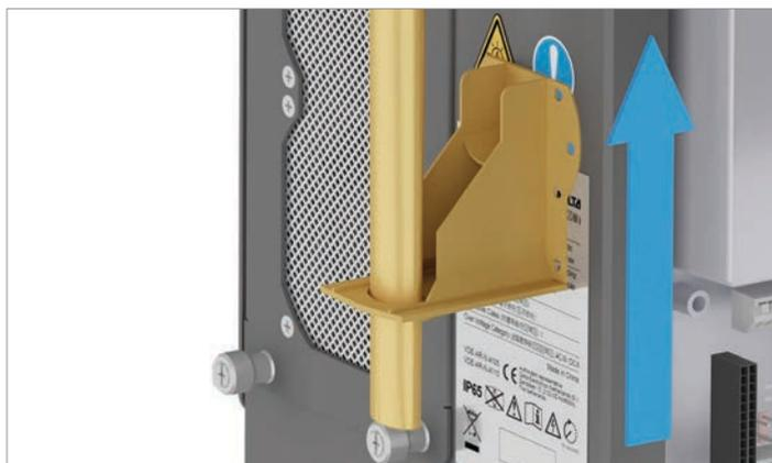
7. Slide the mounting frame over the Sub-1G antenna upside down from below.
