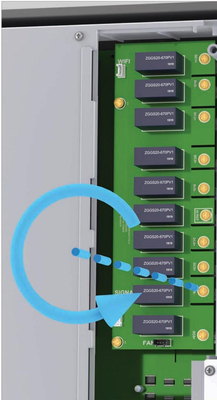
4. Loosen all screws on the printed circuit board with the DC surge protection devices and remove the printed circuit board.
