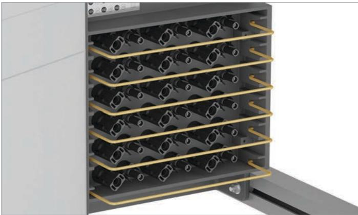
2. Insert the metal brackets to support the DC cables.
