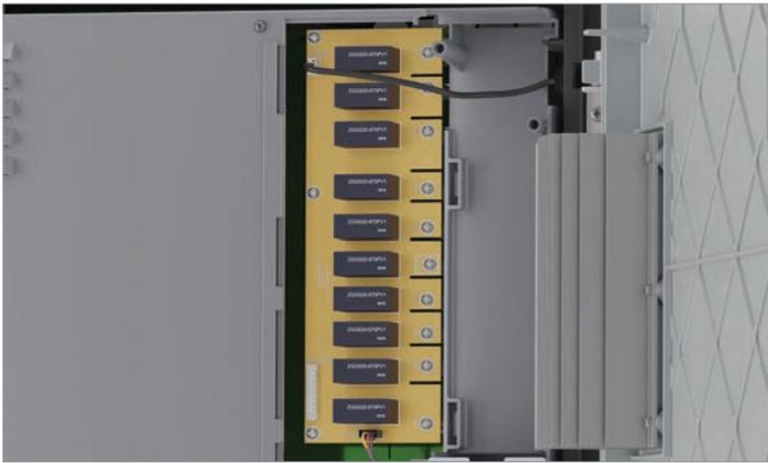
Fig. 4.11: Position of the type 2 DC surge protection devices with the cover removed
