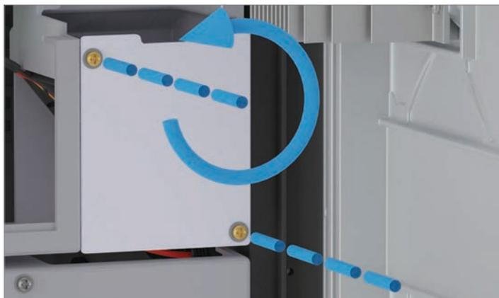
3. Unscrew and pull out the cover. The fan is screwed onto the cover.
