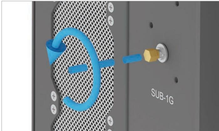
1. Unscrew and remove the cover cap of the Sub-1G connector.
