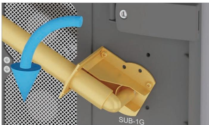
2. Rotate the mounting frame with the Sub-1G antenna downward.
