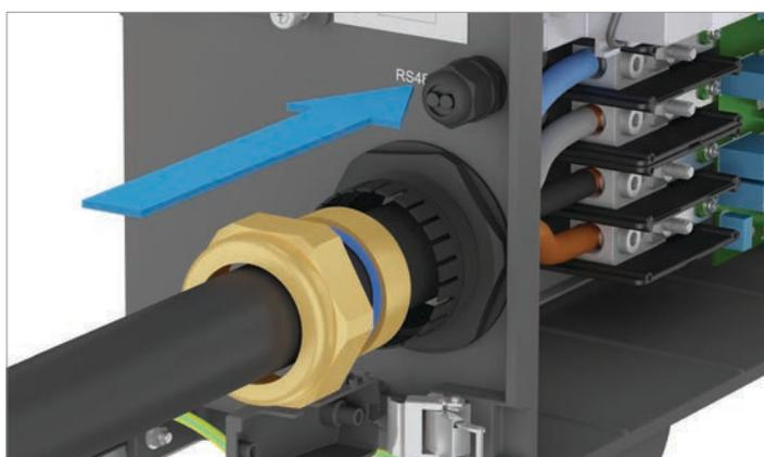
3. Insert the seal and cable gland for the AC connection and screw the cable gland in place.
