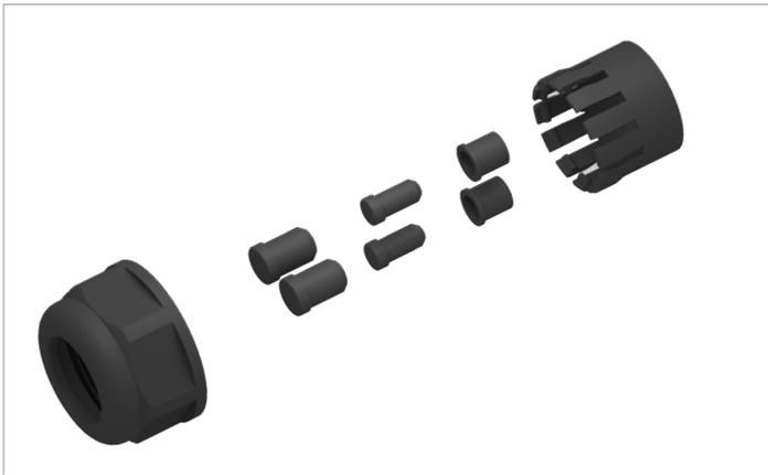
3. Remove the same number of rubber plugs from the seal corresponding to the number of cables to be connected. Do not remove the rubber plugs from the unused seal feed-throughs.
