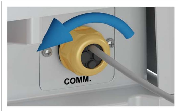
12. Unscrew the cable gland of the communication connection and carefully pull it out slightly.
