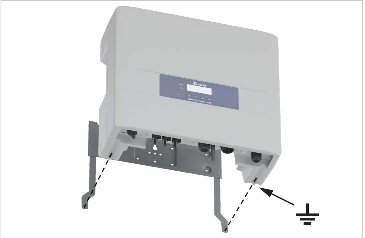
*Fig. 4.9: Location of the mounting holes and the grounding connection on the inverter*
