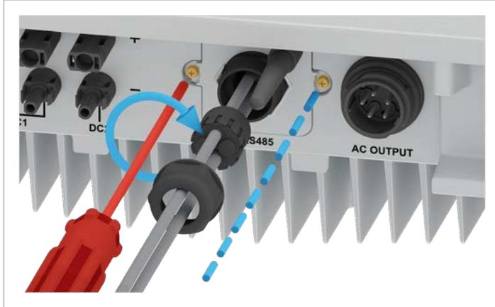
2. Insert the seal and cable gland and screw the cable gland tight.
