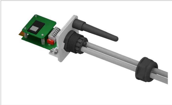
4. Pull the cable through the cable gland and seal.
