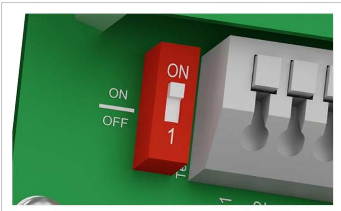
2. Set the DIP switch for the RS485 termination resistor (DIP 1) to the **ON** position.
