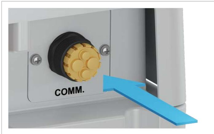
17. Insert the seal and cable gland of the communication connection and fasten the cable gland.
