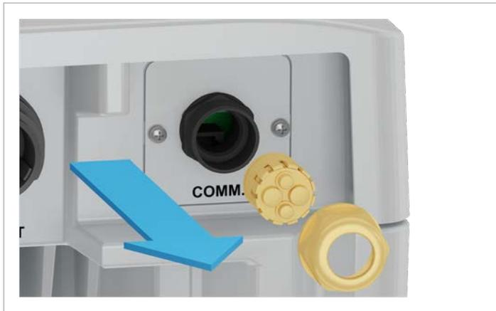
2. Unscrew and remove the cover of the communication connection.
