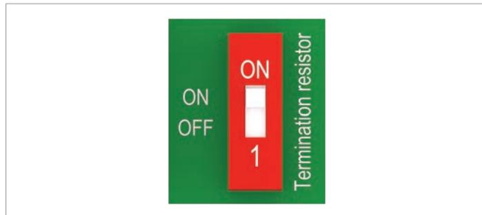
Fig. 6.3: DIP switch for the RS485 termination resistor
