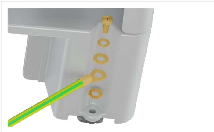
4. Screw the inverter securely onto the mounting plate. Use the screw on the right-hand side to provide additional grounding to the inverter housing.
