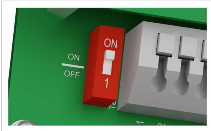
2. Put the DIP switch for the RS485 termination resistor (DIP 1) in the **ON** position.
