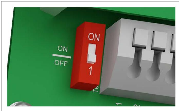
2. Put the DIP switch for the RS485 termination resistor (DIP 1) in the **OFF** position.
