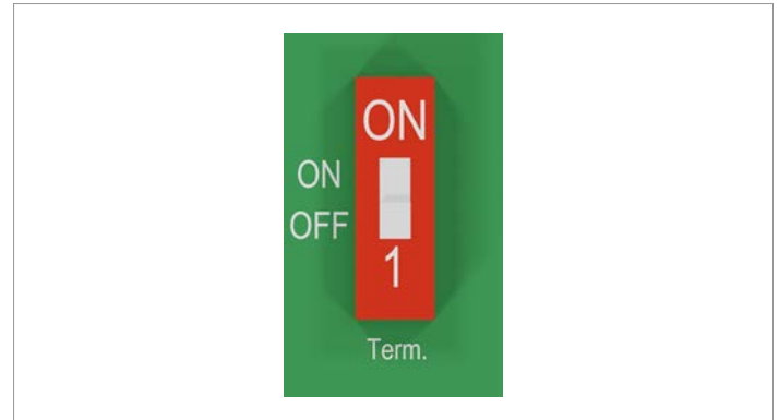
Fig. 7.3: DIP switch for the RS485 termination resistor
