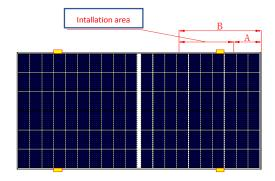
Clamp position can be within the range xxx – xxx mm (clamping range refer to the table below) for all 4 clamps attached to the module long side
