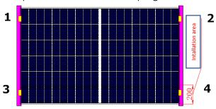
Clamp position can be within the range 0 – xxx mm(clamping range refer to the table below) for all 4 clamps attached to the module short side; clamping range can be asymmetrical, clamp 1&2 can have a different position form the module edge compared to clamp 3 & 4
