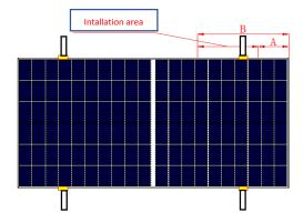
Clamp position can be within the range xxx – xxx mm (clamping range refer to the table below) for all 4 clamps attached to the module long side
