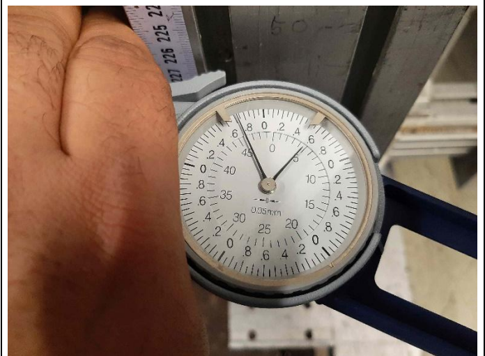
Measurement of glass-package thickness
